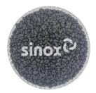
**PCR PP 011304** is a glass fiber filled PP copolymer with increased heat aging stabilization. the Material is suitable for applications with high demands on rigidity at higher temperatures.
